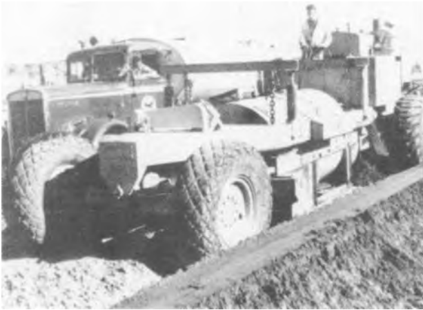
Figure 4-44. Windrowtype pugmill travel plant.
